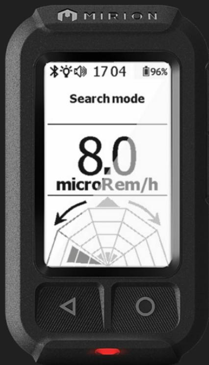
**The AccuRad™ PRD** is a Personal Radiation Detector (PRD) designed for law enforcement, fire and rescue, and other emergency responders to detect and interdict nuclear and radioactive materials. It also provides dose measurement and alarming capabilities for event response.
