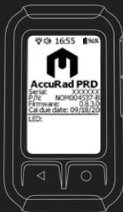
2. Start-up with AccuRad PRD details and self test sequence
